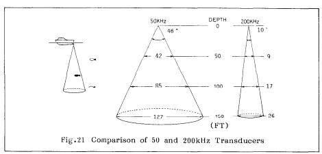
Because the beamwidth of the 200kHz transducer is narrow, the operator has the advantage of higher resolution. In addition, the effects of cruising noise and air bubbles are greatly reduced, since air bubbles resonate at frequencies between 15 and 100kHz. On the minus side, a narrow beamwidth transducer will record even the smoothest bottom contour in a sawtooth pattern if the boat is moving up and down due to pitching and rolling of the boat.
